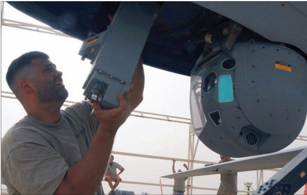
Schuyler Dunn replaces a part of the multispectral targeting system ball on an MQ-1B Predator at Ali Base, Iraq. (USAF photo/Tech. Sgt. Sabrina Johnson.)
