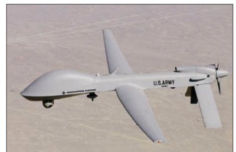
Task Force ODIN forces flew Warrior Alpha UAVs equipped with electrooptical and infrared sensors or with synthetic aperture radar, along with laser target markers, laser rangefinders and missiles.
