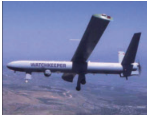
The initial Watchkeeper platform is based on Elbit Systems' Hermes 450 UAV platform.
