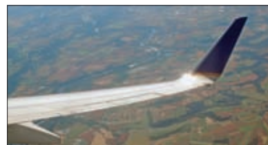
Although winglets are being considered for future aircraft, retrofitting would not be cost-effective.
