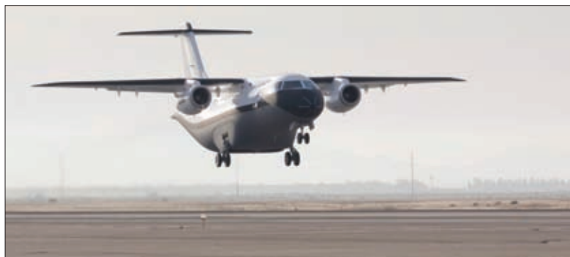
The Advanced Composite Cargo Aircraft is a proof of concept technology demonstrator for advanced composite manufacturing processes in a full-scale, certified aircraft. It was developed by AFRL and Lockheed Martin officials.
